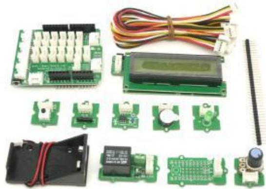
The grove system components include close to a hundred sensors and actuators, which all connect thru 4-position cables from the component to the CUI32Stem -- no soldering.
