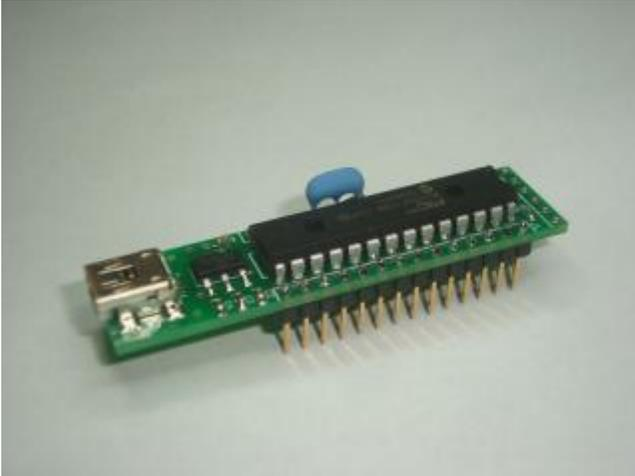
The minimum introduction with "easy assembly" kit includes everything above, and the PIC32MX250F128B on a small pre-assembled PCB with the USB connector and regulator already soldered on, 8MHz resonator, as well as the following components:
